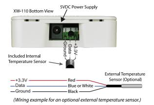
**Note:** The XW-110B only supports 1 temperature sensor. If an external sensor is used, the internal sensor must be removed.
